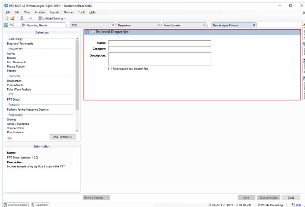
To add a detector to the protocol, choose detector from list of **Detectors** and select **Add Detector >>** **General Properties** and the **Input Signal** can be edited.
