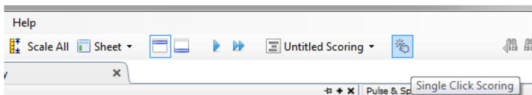
Within the applicable signal sheet manually score an event on the relevant signal trace, for instructions on how to manually score an event refer to the *Scoring an Event* section above. When you have scored the first event the single click scoring feature will enable you to continue scoring the same event type with only single mouse click as you browse through the recording.
