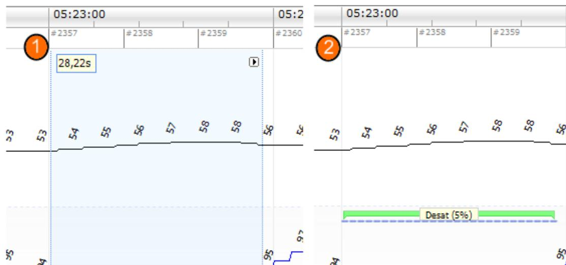
An alternative method for scoring an event is to highlight an area with the left mouse button, as before, but then right-click on the area and select an event from the list.
