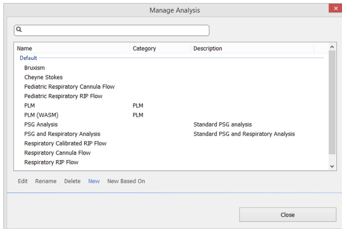
For this example we will create a new analysis protocol. Select **New** in the **Manage Analysis dialog**. A new **Analysis Protocol** sheet will open up where the new protocol can be defined. A protocol is a collection of detectors and the function of a detector is to locate areas of interest within a signal and score the areas with events.
