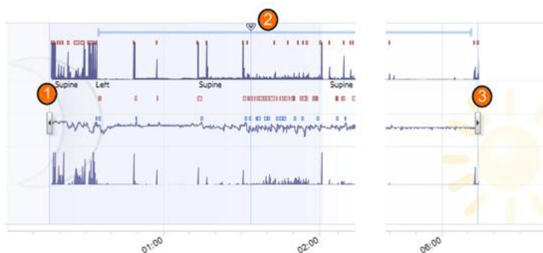
To navigate into the recording use the synchronization marker **2**. All signal sheets such as the **PSG**, **Respiratory** and **Pulse Oximeter** sheets are synchronized accordingly. If an interesting event is located in the overview, drag the synchronization marker over that area and browse into the relevant signal sheet to view the raw signals.
