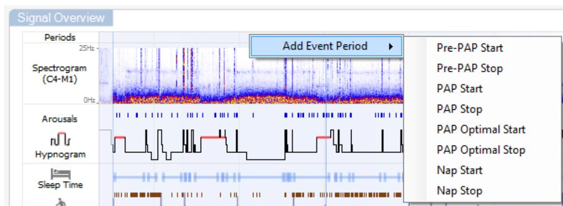
Sleep scoring and exclusion of invalid data can be performed in Signal Overview panel. To score sleep or exclude invalid data from the recording locate the mouse pointer to the **Periods** panel, left mouse click and select an area by dragging left/right. Release the mouse button and the menu showed below will be available. The 'Awake' events and 'Invalid Data' events will be excluded from the report calculations.
