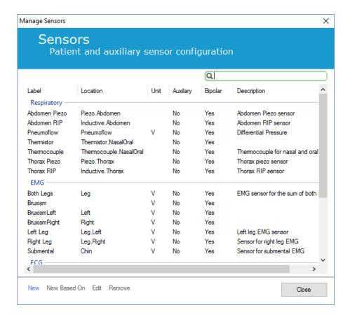
You can select whether a new patient sensor or an auxiliary device sensor is to be created. Fill in the applicable fields and click **OK** to save the sensor configuration.
