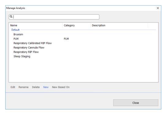
For this example, we will create a new analysis protocol. Select **New** in the **Manage Analysis dialog.** A new **Analysis Protocol** sheet will open up where the new protocol can be defined. A protocol is a collection of detectors and the function of a detector is to locate areas of interest within a signal and score the areas with events.
