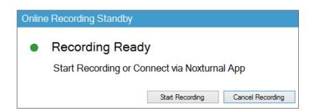
When the user has connected the Noxturnal App to the online room the live traces that start to appear are **NOT** being saved to the recording. It is only a preview as is indicated by the preview status. The signal will start to record as soon as the user hits **Start Recording** either in the Noxturnal App or in the Noxturnal US software.
