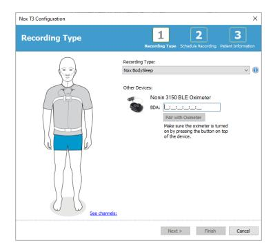
If your Recording Type is set up to record data from an auxiliary Bluetooth device, e.g. pulse oximeter you will see that in the Configuration Wizard. To be able to use auxiliary Bluetooth device it needs to be paired to the Nox recording device. Enter the appropriate Bluetooth device Pin/BDA (Bluetooth Device Address) number in the relevant field in the Configuration Wizard.
