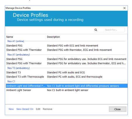
To create a custom device profile, select New or New Based On. You will then need to select for which recording device the template is for or from which of the current device profiles you wish to base your new template on. For this example, we will create a new device profile for the Nox T3 Recorder.
